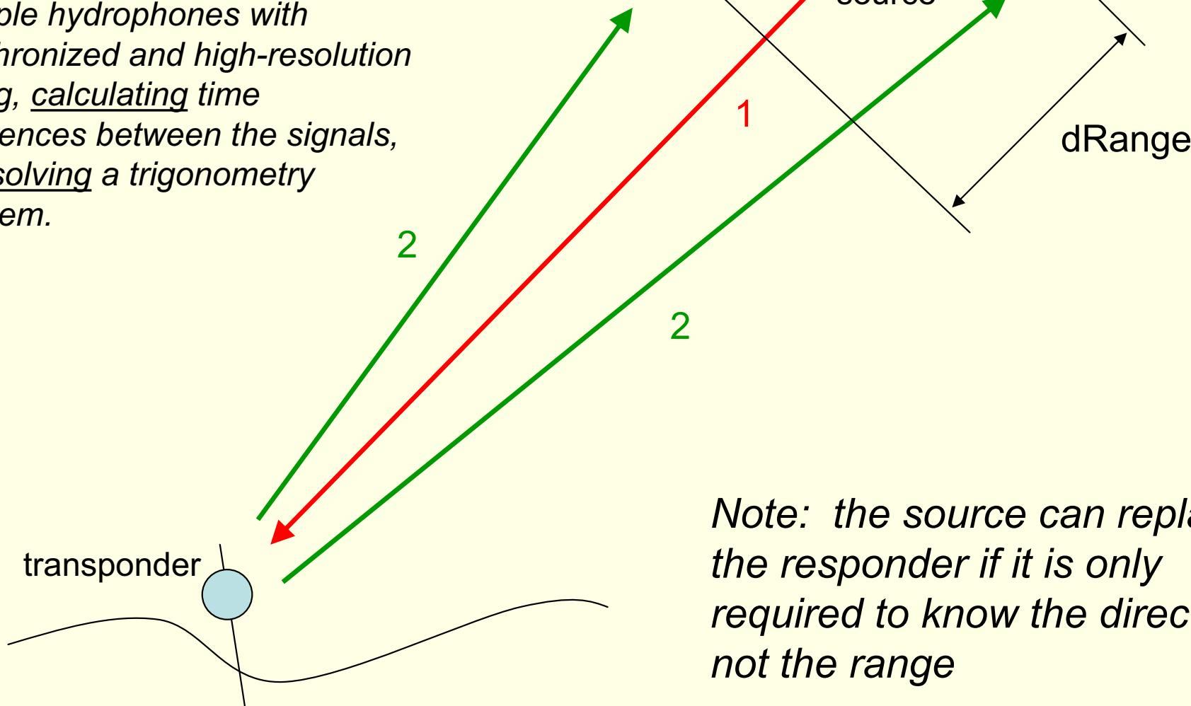
Note: the source can replace the responder if it is only required to know the direction, not the range
